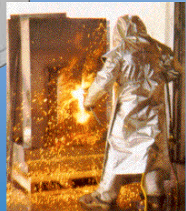
Technician attacks a Hamilton Vault Panel during a fiery U.L. rating test.
